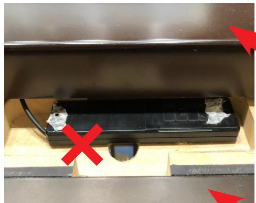
Drill hole Not sufficient when Metal is close.
