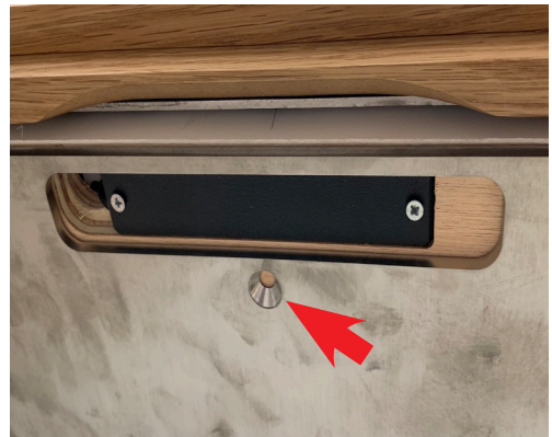
Metal near the reader may block or reflect the signal, causing key/card reading failures.
